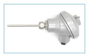
have insulated junctions to prevent earth loops. The metal sheaths are impervious to liquids and gases and can withstand high pressures. The diameters range between 3.0mm up to 8.0mm and the sensors can be formed to shape particular applications without impairing performance. The typical bending radius is 10 x probe diameter but can be reduced to 4 x if required.
